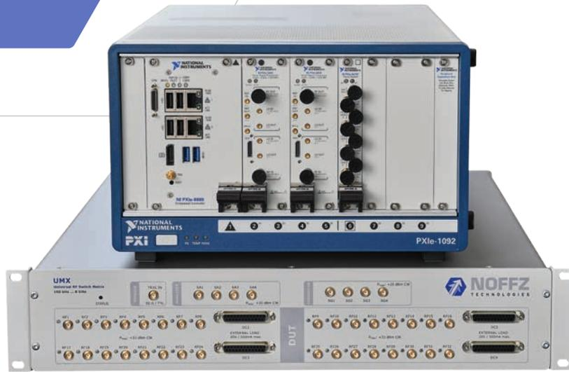
UWT configuration with 2 RF transceivers, 32-port UMX and additional PXI instruments
