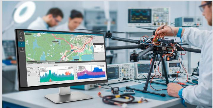
It supports differential GNSS and multi-vehicle simulation, GNSS satellite orbit modification, unlimited pseudorange additive ramps and custom fixed positions. Available in Single/Dual/Triple Band hardware configurations, add jamming for detailed interference validation for low-latency HIL applications.
